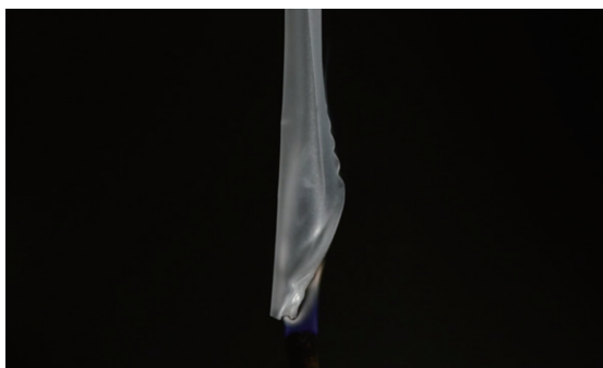
6% loading to PP (100 \mu m VTM-0)
